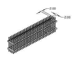
MMT Machrone also offer a special 2.0mm stacker for PC104 + stack through application.
